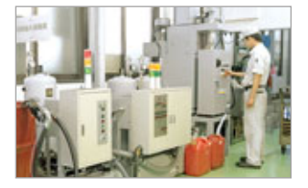
Wasted production oil is 97% recycled after being purified via special filtration equipment.
